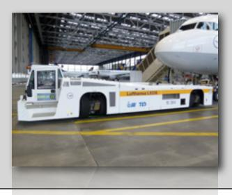
The hybrid-electric aircraft tractor that can be controlled by a pilot is being used by Lufthansa Technik's subsidiary Lufthansa LEOS to tow aircraft between the gate and the runway. Using the Taxibot, aircraft can be taxied with their engines turned off, which reduces fuel costs and airport carbon emissions, as well as eliminate bottlenecks in the gate area.
